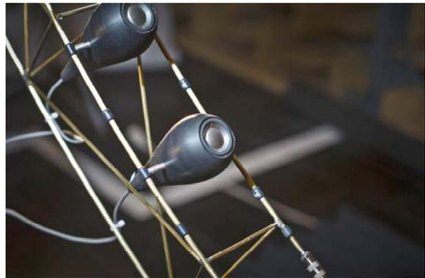
**Figure 1 – Developed drop-like loudspeaker with mounting to the arc.**
