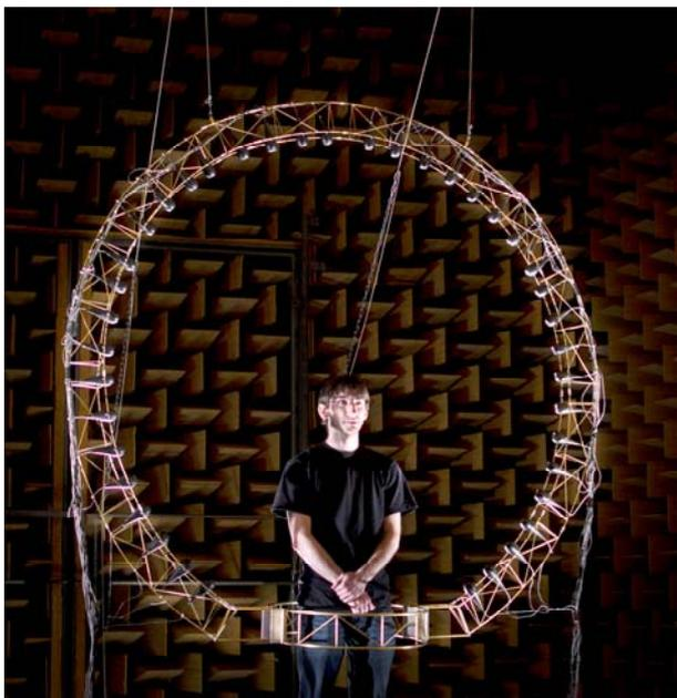
**Figure 3 – Measurement of the individual HRTF of a subject.**
